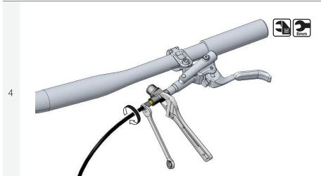
Tighten connecting bolt using 8mm spanner while pushing the brake hose into OutBraker body.
