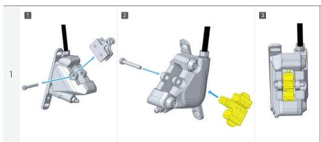
Remove the brake pad and install bleed spacer in the caliper.
