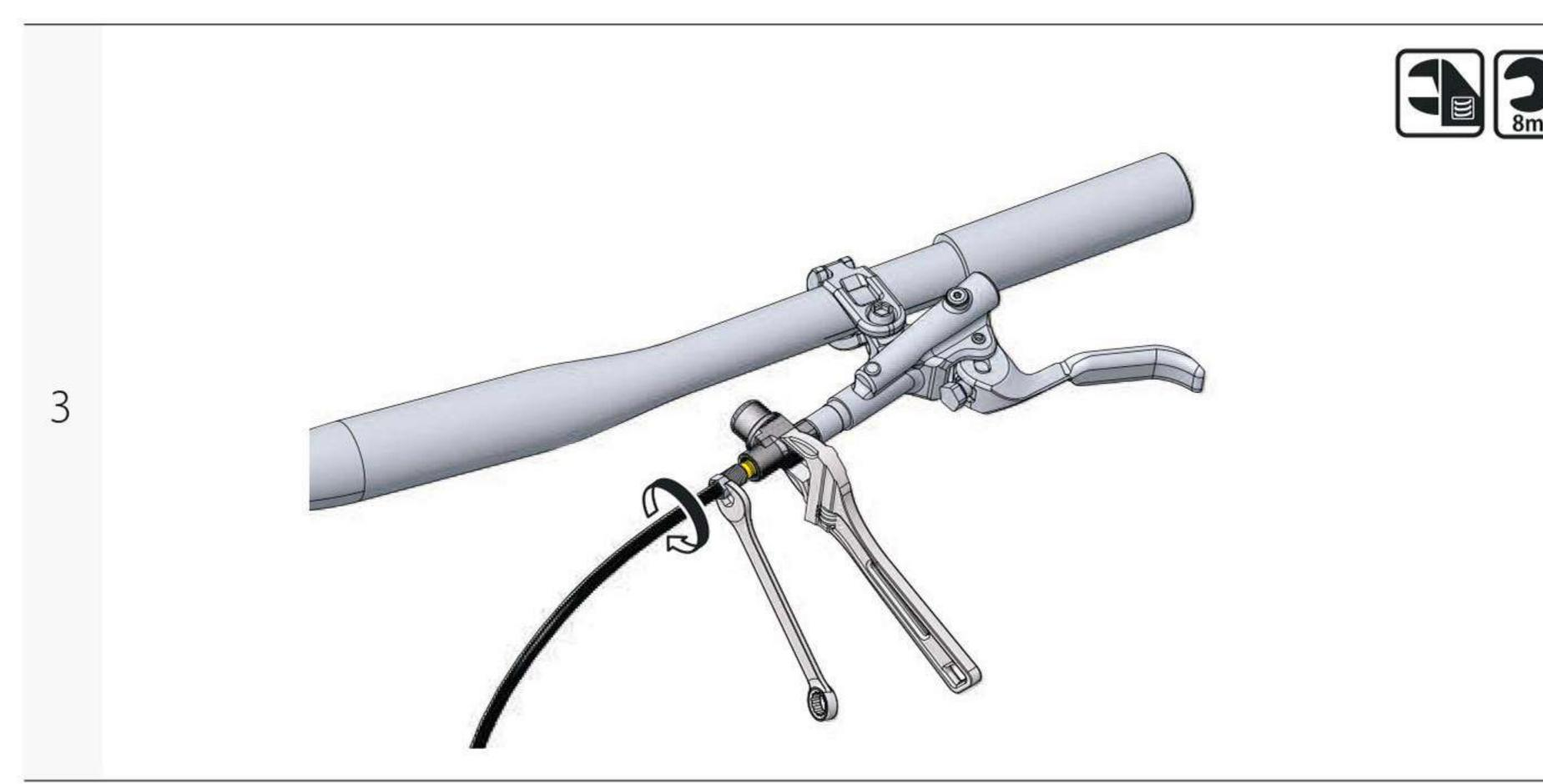
Tighten connecting bolt using 8mm spanner while pushing the brake hose into OutBraker body.
