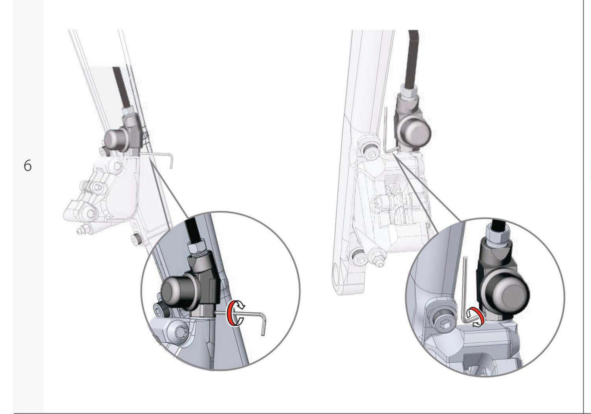
Fix the angle using the hexagonal wrench included.
